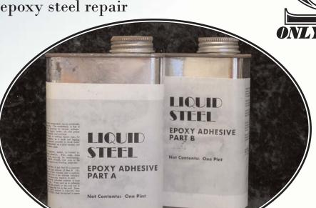
LIQUID STEEL is a 100% solid, two-component, epoxy-polyamide cured system that is highly resistant to water, oil, grease, and solvents. LIQUID STEEL will bond steel to steel and to concrete. It is ideal for a caulk and lagging compound as well as for attaching electrical boxes to poured concrete or block walls, making drilling unnecessary. Can also be used as a joint sealant and patching compound in low pressure water and sewer pipes.
